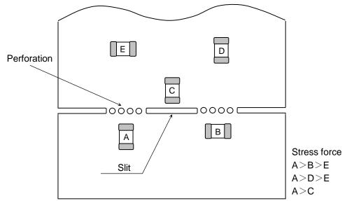
When dividing printed wiring boards, the intensities of mechanical stress applied to capacitors are different according to each dividing method in the order of:
