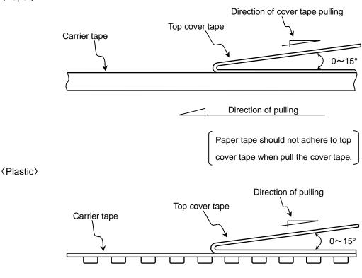
3-2. Carrier tape shall be flexible enough to be wound around a minimum radius of 30mm with components in tape.
