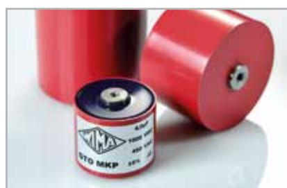
**GTO MKP Capacitors for Pulse Applications with Internal Series Connection. Capacitances from 1.0 µF to 100 µF. Rated Voltages from 400 VDC to 2000 VDC.**
